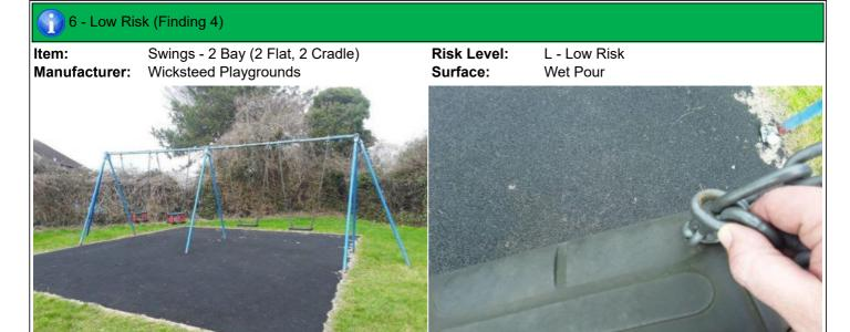
**Action:** Monitor for any further deterioration and replace when 40% worn
