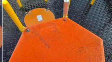
**Finding:** There is/are finger entrapment/s in the seat and the item fails to meet the requirements of BS EN 1176 Part 1 4.2.7.6 Entrapment of fingers
