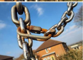
**Finding:** A number of fixing(s) have worked loose (hand-tightened on-site)
