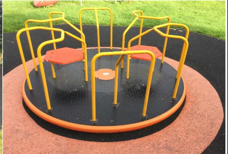
**Finding:** There is wear in the bearing/shaft causing some movement?
